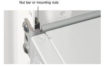
**10** Push the server toward the back of the cabinet until the front of the server rails touch the front cabinet posts, then secure with two screws through each server rail.
